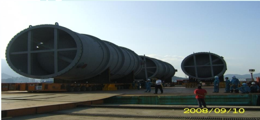
Loading Beam / 13.2m x 2.0m x 1.0m (Longest) Shipped on a Ro-Ro vessel with an evaporator for local transportation to job site.
